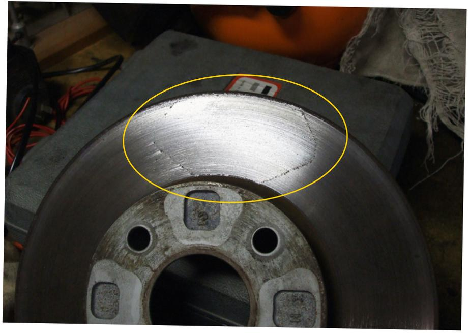
practice not to jam on the hand brake while the brakes are hot (whether after a stint on the track or on a Club run), as this constrains the discs from moving while cooling and can also result in the pads being “welded” to the disc, due to the combination of heat and pressure.
