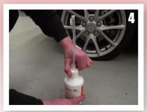
Remove cap from the bottle, and screw on the injection hose with the bottle's inner cap left on to break the inner cap.
