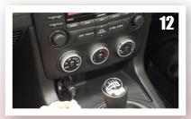
Insert the compressor plug into the interior accessory socket and turn the ignition switch to the ACC position.
