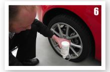
Remove the plug from the injection hose and insert hose on to the valve.
