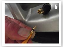
Remove the valve cap from the flat tyre. Press the back of a valve core tool to the core of the tyre valve and bleed all the remaining air. Turn the valve core anti-clockwise to remove.
