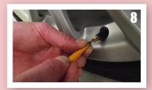
Remove the injection hose from the valve. Reinsert the valve core into the valve, and turn it clockwise to install it.
