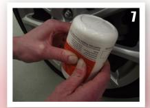
Hold the bottom of the bottle upright, squeeze bottle with your hands, and inject all of the tyre sealant into the tyre.
