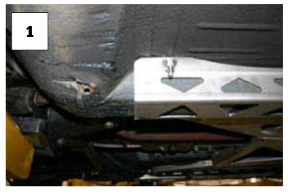
Positioning the frame rails. Photo: Flyin' Miata
