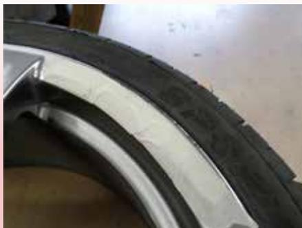
*Mask around the damaged area ...*
