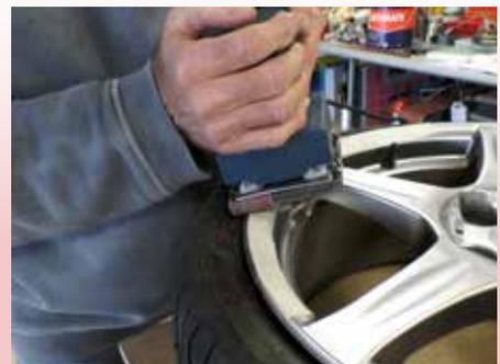
*Carefully sand out the damaged areas ...*
