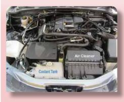
Loosen the two clamps holding the rubber hose between the air cleaner and the inlet manifold.
