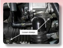
Undo the two clips holding the air cleaner box together.
