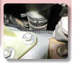
If the rubbing is severe, it would require the various radiator hoses to be loosened and repositioned to align the pipe in the correct position.
