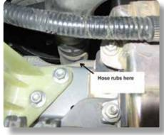
Repositioning the hose in the large white nylon clip won't permanently move the pipe as the clip doesn't holds the hose securely which is why it squeaks.
