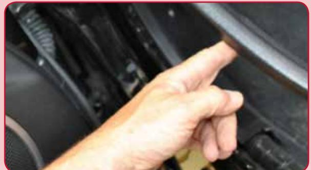
3. Remove the plastic rivet under the internal fuse box cover/kick panel.
