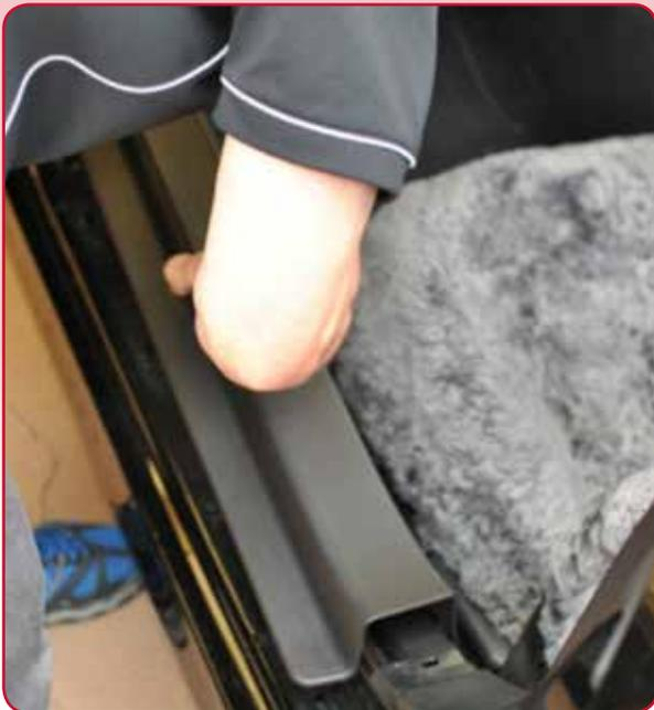
2. Pull away the rubber door seal up to the dash vent.
