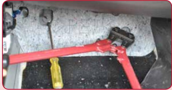
5. Remove the trim fastener holding the carpet in place.
