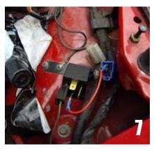
Then make another wire for the earth/chassis connection at the relay.
