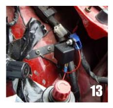
All that's left to do now is cross your fingers and give it a test beep! Remember that the car ignition will need to be switched to the on position when you do this, as the blue plug is not constantly live. Hopefully when you hit the horn button you'll be greeted with a healthy blast of noise. It's not ear-splittingly loud, but it is certainly a vast improvement on the standard item.
