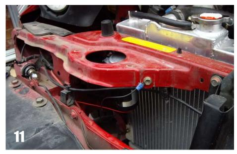
When mounting the horn, you might need to jiggle and manoeuvre the bracket and horn around a bit to get it into perfect position, so don't do any of the bolts up super tight just yet.
