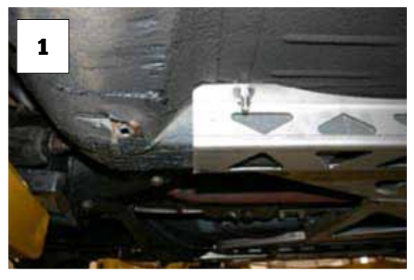
Positioning the frame rails. Photo: Flyin' Miata
