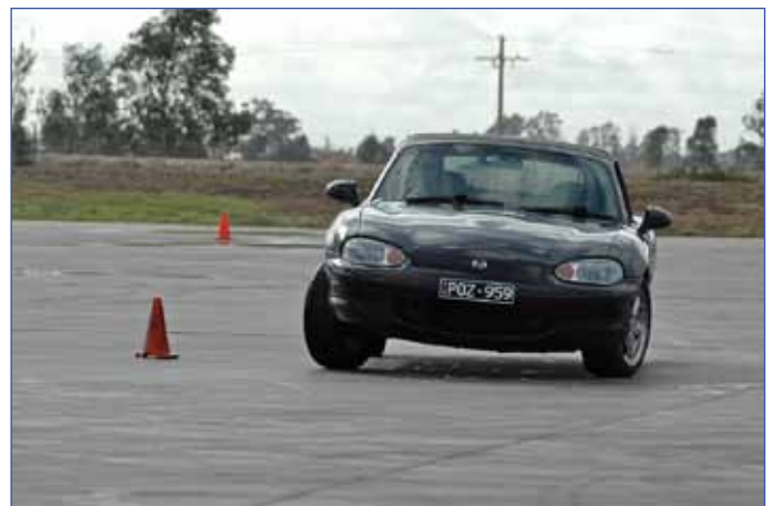
Figure 5 - Weight transfer to the left tyres decreases the grip of the right tyres. With an open differential it would be easy to spin the inside rear wheel under power
