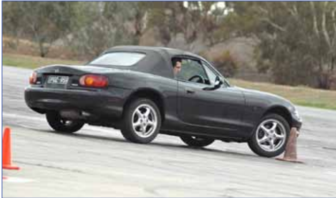
Figure 6 - Handbrake turn initiated, now the power has been applied to keep the slide going
