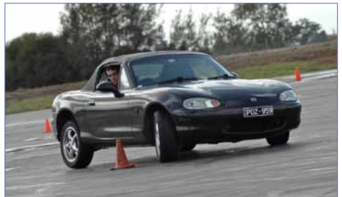
Figure 7 - Keep it close to the cones! Also, note the weight transfer to the front end due to braking. This will make it easier to initiate the handbrake turn necessary to get the back tyres around the cone.
