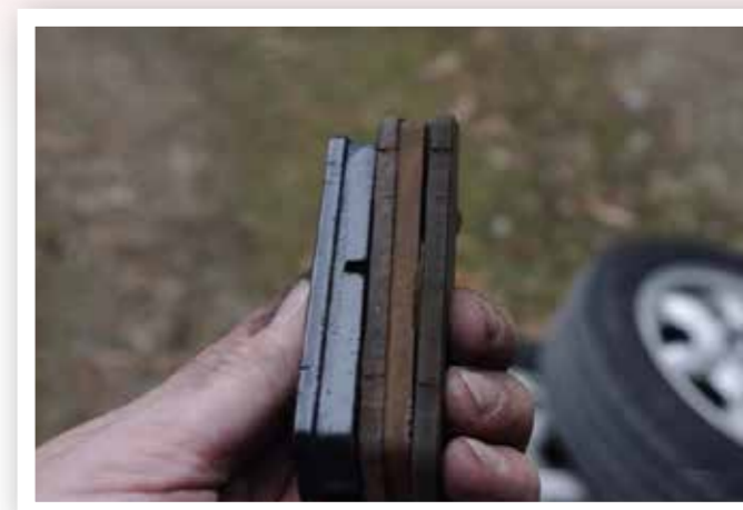
From the top: new pad, outer pad and inside pad. Note the difference in thickness between the old pads. Not good!
