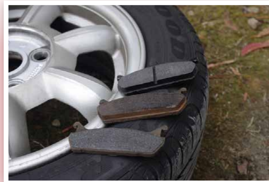
From the top: new pad, outer pad and inside pad. Note the difference in thickness between the old pads. Not good!
