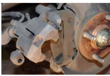
After removal of the sliding pin, the caliper can be rotated upwards away from the disc so that the old pads can be removed
