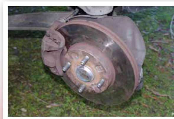
Front caliper and disk, the shield allow more clearance.
