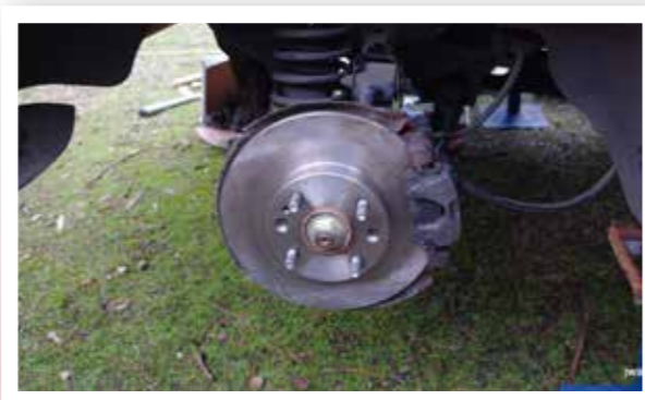
Disk, showing the adapted dust shield. Note the places where the shield is cut which allows it to be bent.
