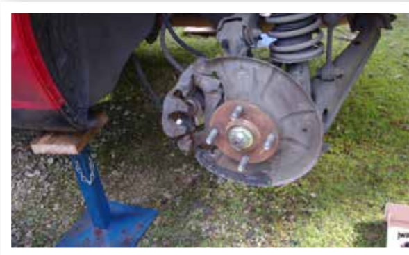
Old caliper still in place, disk shield clearly visible. Some crimping of the shield can be seen.
