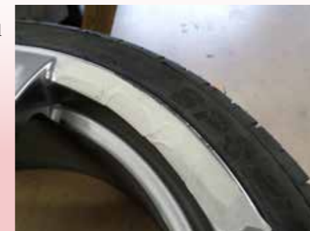
Mask around the damaged area ...
