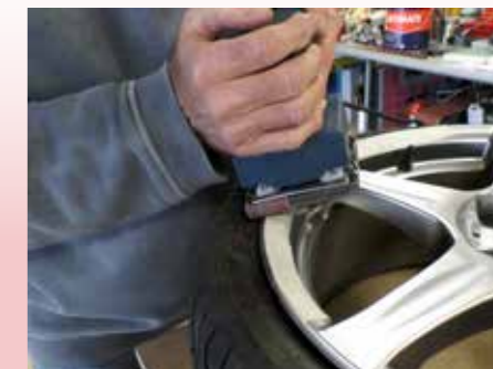
Carefully sand out the damaged areas ...
