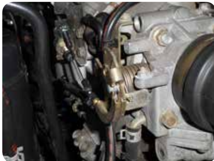
Cruise control cable looped over original throttle cable barrel
