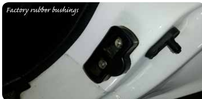
Use a 10mm socket to remove the old fixing bolts.
