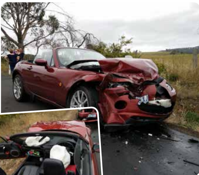
It's crumpled, but that's how it's designed: the body absorbs the energy and protects the occupants
