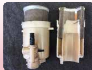
The Fuel Pump Housing AND High-Pressure Filter
